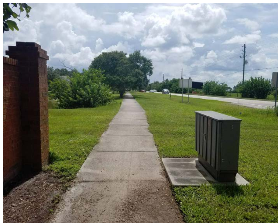
North side of Partin Settlement Road existing constraints. The trail may fork in this location to provide two 6ft wide paths in lieu of relocating the utility box.
