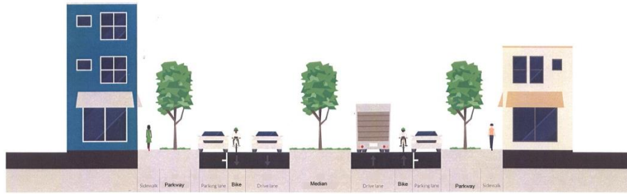
Figure 5: Four-Lane Avenue/Boulevard with Turn Lane/Median
