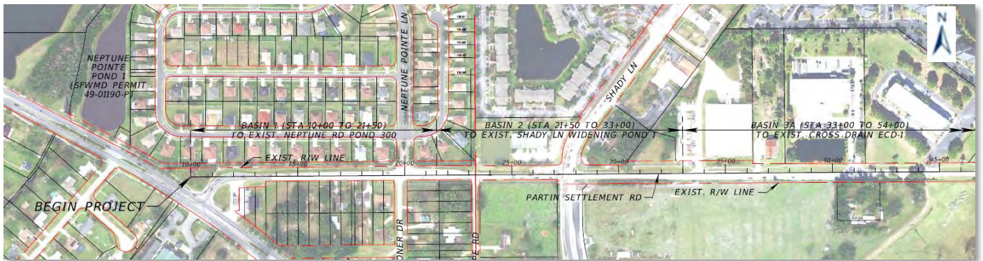
Figure 3: Drainage Basin Map - Basins 1, 2, 3A
