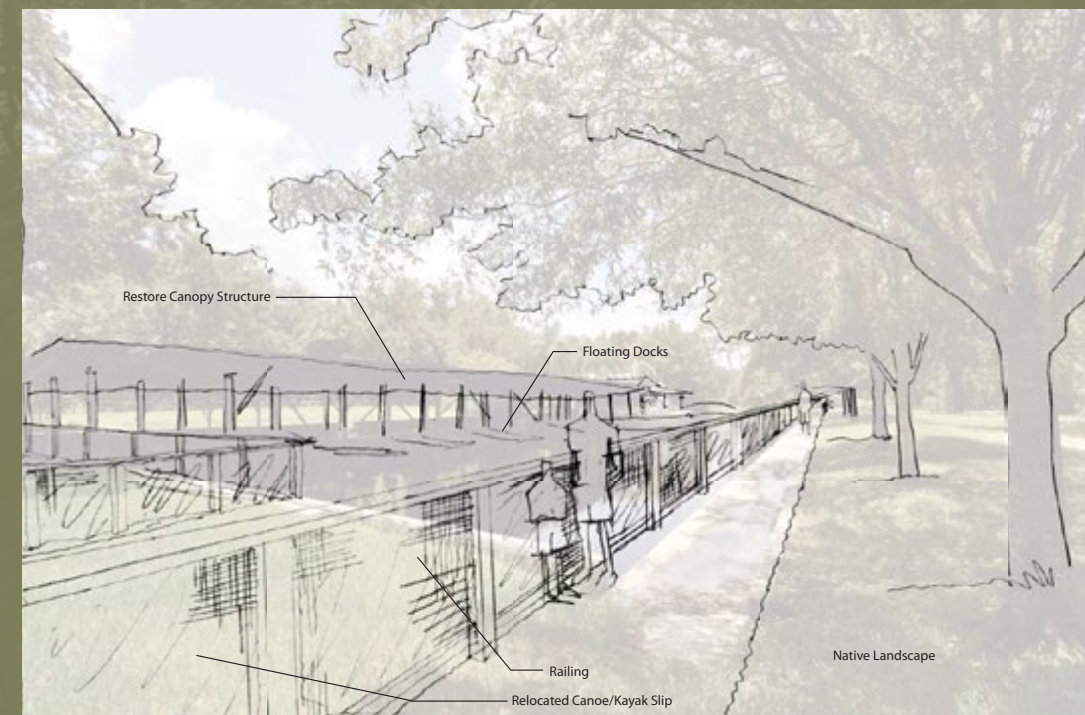
Existing boat basin preserved and fenced for safety. Existing boat shelter restored with new floating docks installed for electric boats and canoe/ kayaks.
