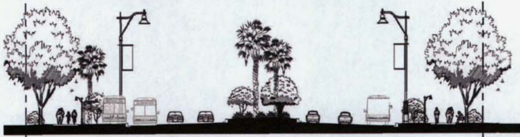
Example Multimodal Roadway Design (Urban Section)
